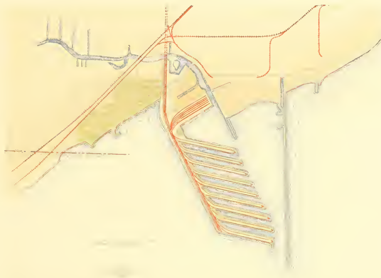
LXXII. CHICAGO. SKETCH DIAGRAM OF DOCKS SUGGESTED AT THE MOUTH OF THE CALUMET RIVER FOR BULK FREIGHT STEAMERS; ACCESS TO BE HAD WITHOUT OPENING OF BRIDGES.
